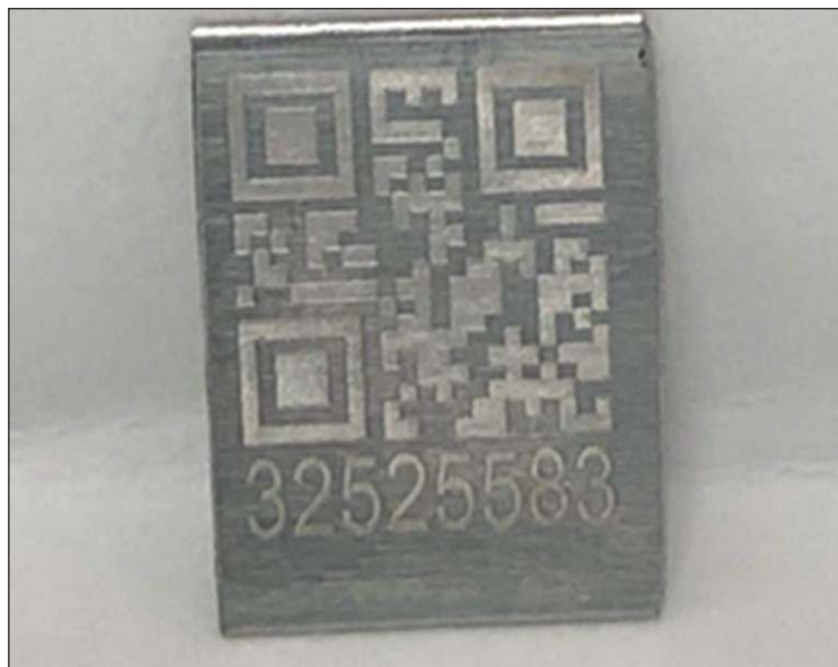
Figure 1: QR code and DNI number engraved by laser.
